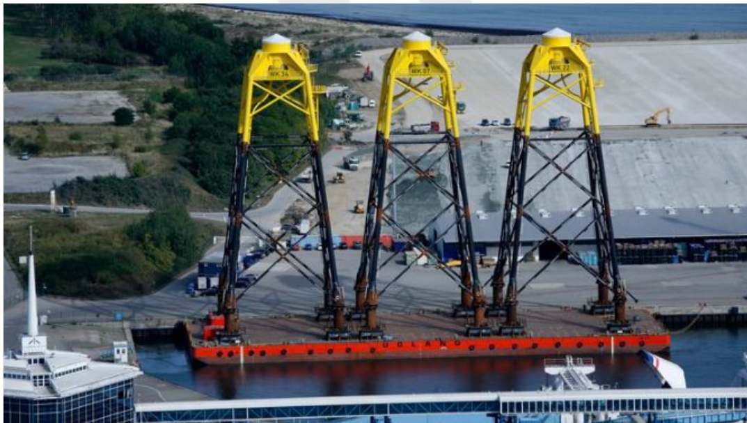
Figure 2-4: Jacket Structures for the Wiking Offshore Wind Farm [12]
